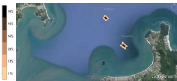
Figure 8 : Exceedance frequencies of BOD concentrations for two scenarios with different outfall lengths for pre-treated wastewater discharging at Canasvieiras.
